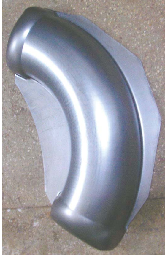
Fig. – General view of semi-product of half-pipe with diameter 200 mm made of carbon steel 08kp of sheet thickness 1.2 mm
